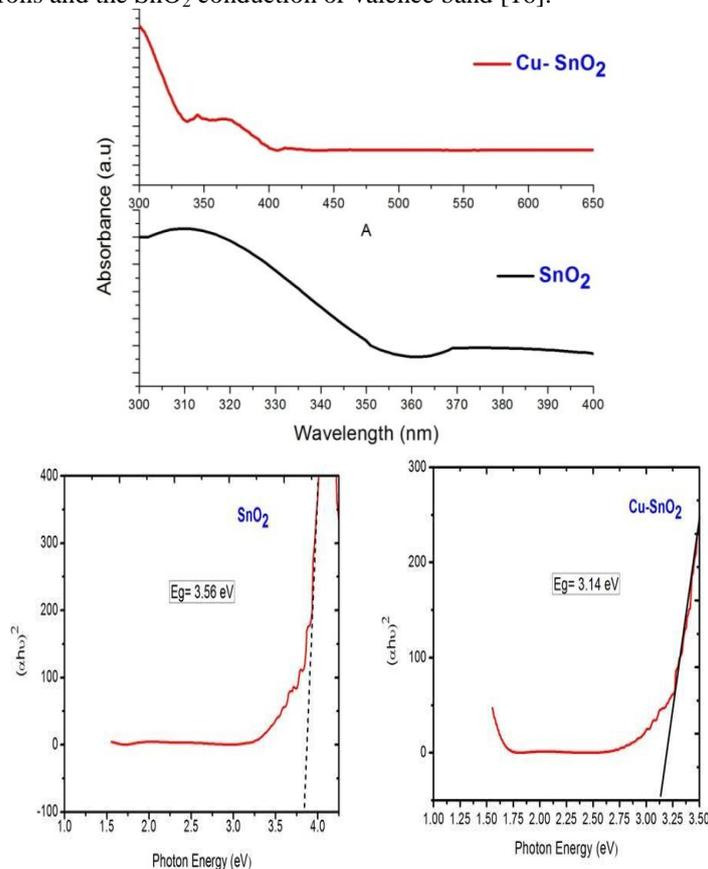
Fig 3. UV-DRS Spectra and Fig 4. K-M plots of pure and plasmon assisted SnO<sub>2</sub> nanoparticles
