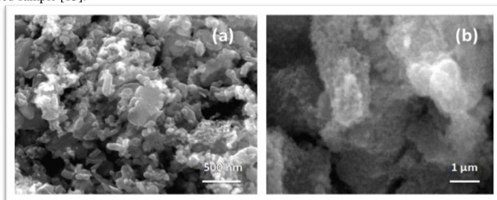
Fig 2. FESEM micrographs of pure and plasmon assisted SnO<sub>2</sub> nanoparticles
