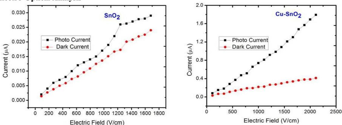
Fig 6. Field dependent dark and photocurrent plots of pure and plasmon assisted SnO<sub>2</sub> nanoparticles
