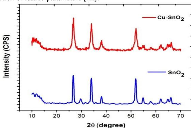
Fig 1. XRD patterns of pure and plasmon assisted SnO<sub>2</sub> nanoparticles
