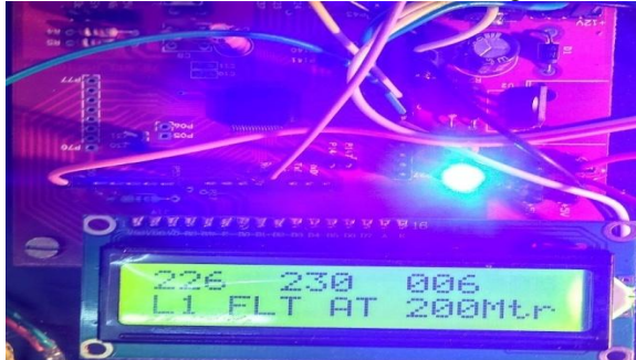
Fig.4.2 fault at line 1
