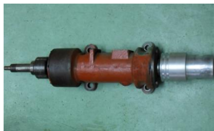
Fig. 4. Spindle with its bearing units
