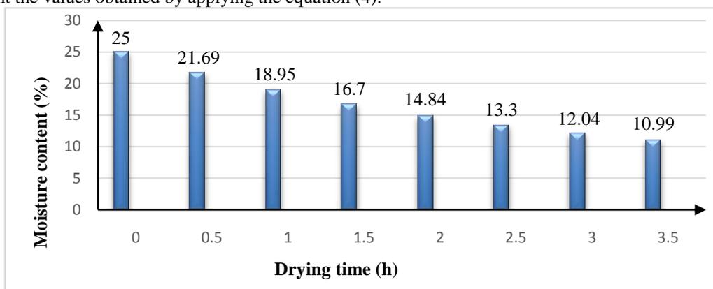
Fig.5 : Variation of the moisture content with the drying time
