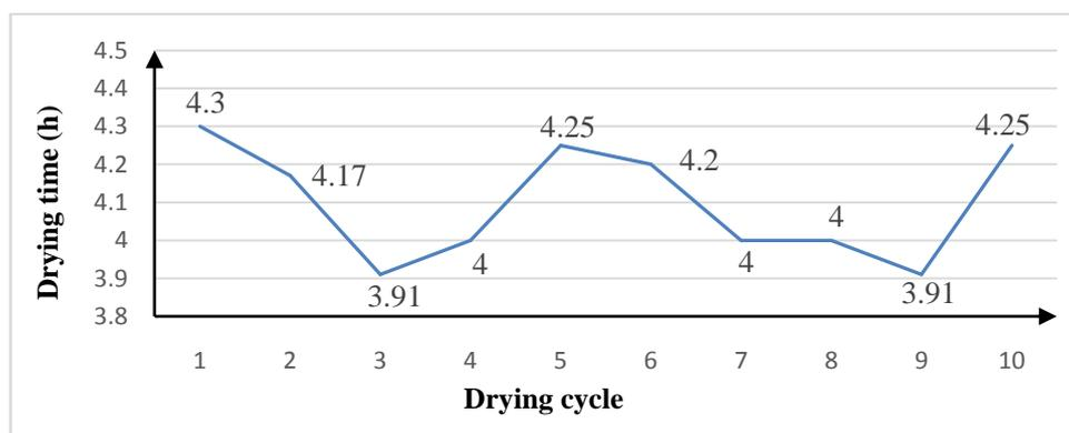
Fig.6 : Drying time for ten drying cycle with manual stirring
