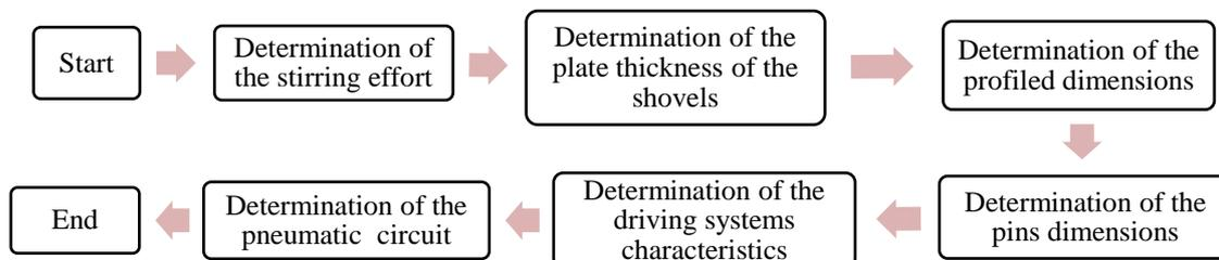
Fig. 3 : Machine sizing algorithm
