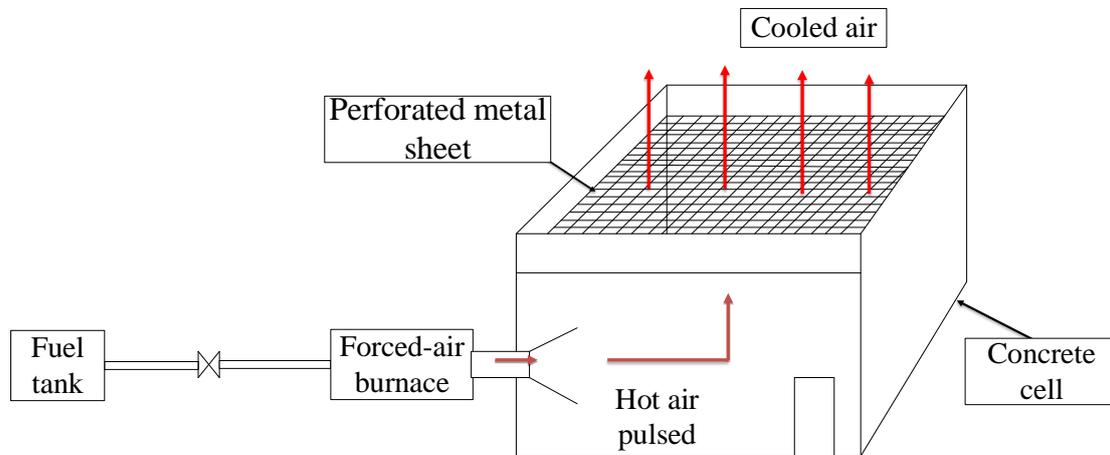
Fig. 1: Description of a drying unit
