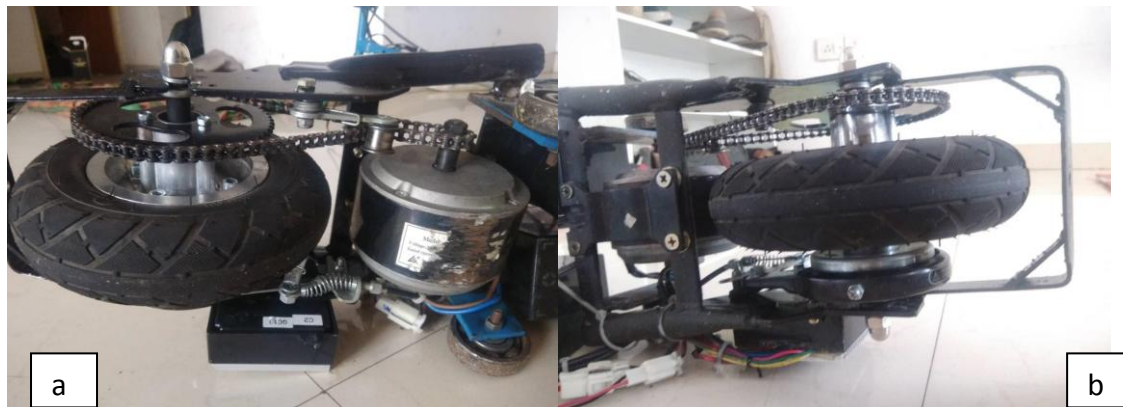
Figure 6. Typical Assemblies, a) Motor with chain drive, b) Sprocket wheel
