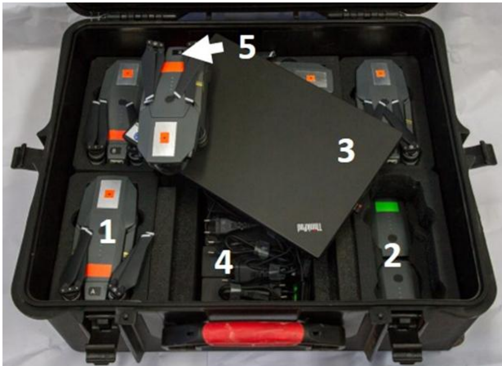
Figure 1:Photogrammetry Swarm Transport Container: (1) Five UAVs-model DJI MP; (2) Ten spare batteries; (3) Notebook computer; (4) Battery charger & spare parts; (5) Tape,
