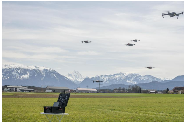
Figure 4: Photogrammetry Swarm in action, with five MP drones in swarm formation hovering above the transport container during a test flight in 2018; a sixth drone is filming the swarm.
