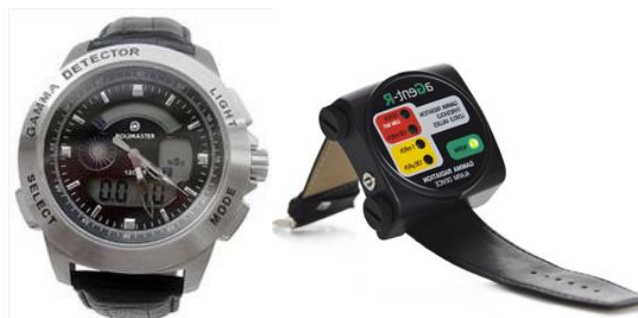
Fig. 10 Wrist watches as gamma dosimeter (left) and warning device (right; POLIMASTER, Gamma Radiation Dosimeter; http://shop.polimaster.us/pm1208m-wrist-gamma-indicator-radiation-detector/ )
