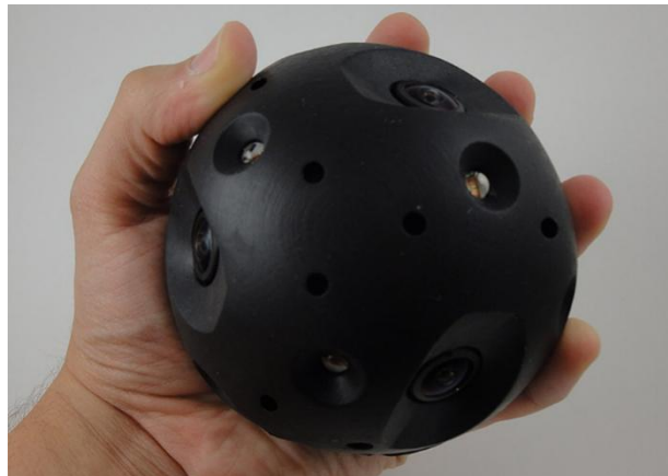
Fig. 9 Camera ball with six-lenses for 360 degree coverage (Bounce Imaging Explorer, https://www.bounceimaging.com/ ; last accessed 30 August 2018)
