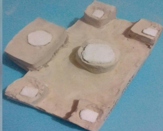
Fig 3: Plate shell formed and left for drying
