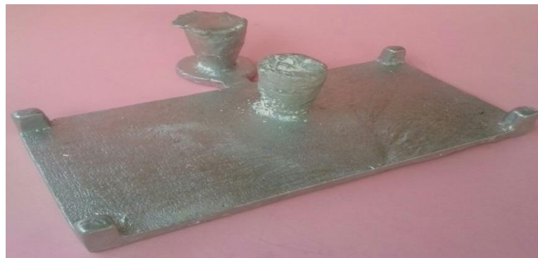
Fig. 7: Plate obtained after knockout operation
