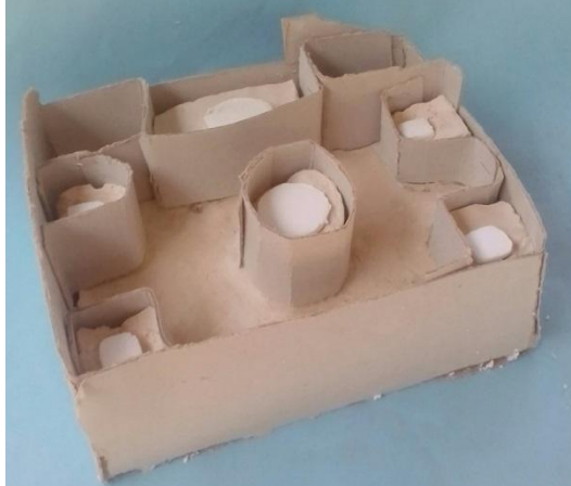
Fig 2: Strawboard box temporarily housing the pattern and the poured slurry
