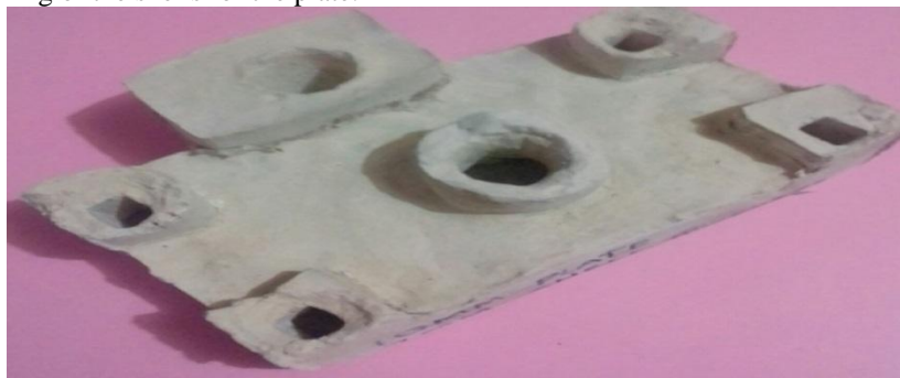
Fig 4: Shell produced after burning of polystyrene and firing
