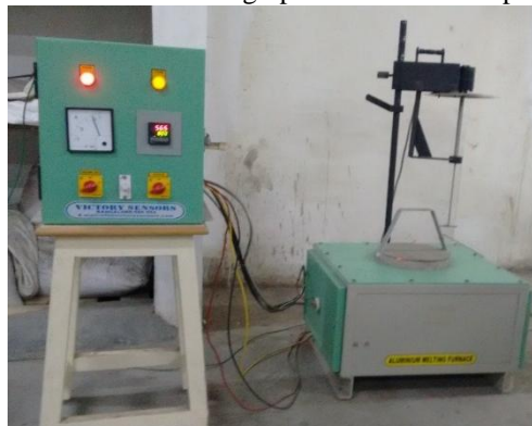
Figure 2 Stir casting setup with furnace
