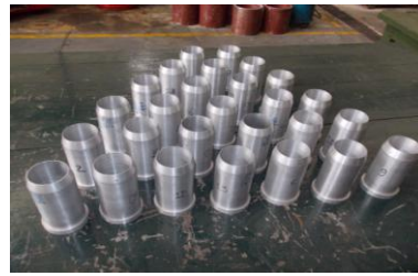
Fig. 3b Machined Preform before forming
