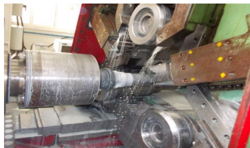
Fig. 2 The flow forming machine (Three – Rollers)
