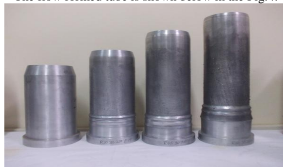
Fig.4 flow formed tube with 30%, 45%, and 60% of reduction
