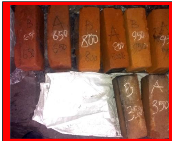
Plate 1.0: Variation in the colour of brick with firing temperature
