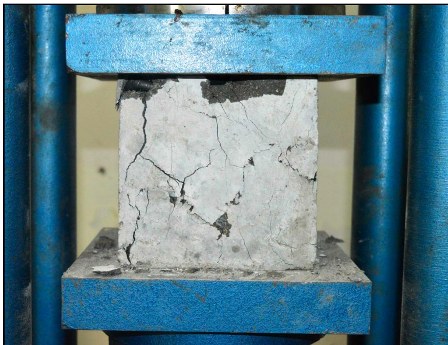
Fig 4.3: specimen after failure
