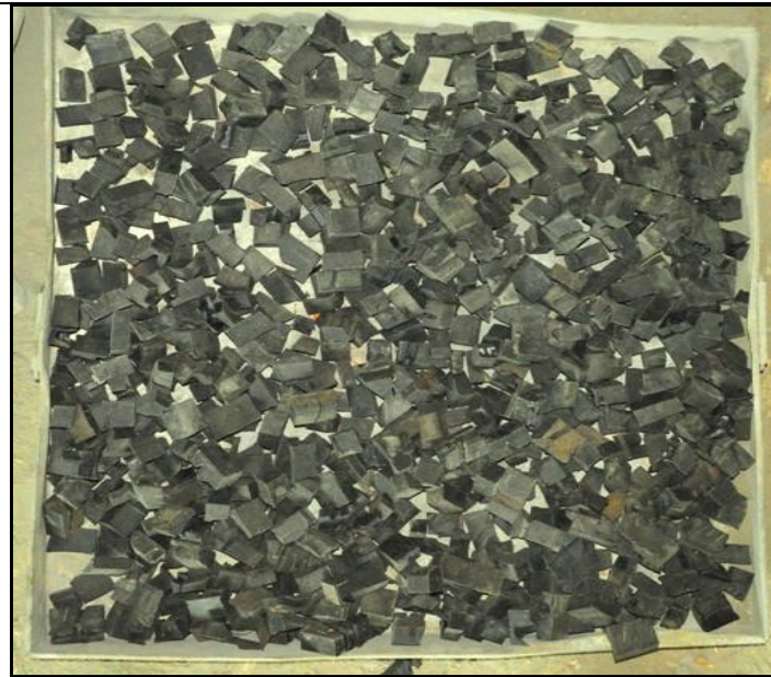
Fig 2.3: Chipped Rubber Samples
