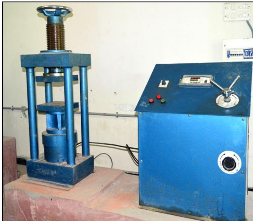
Fig 4.2: compressive test machine
