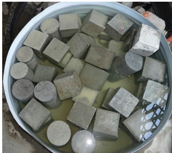
Fig 4.6: water curing tank
