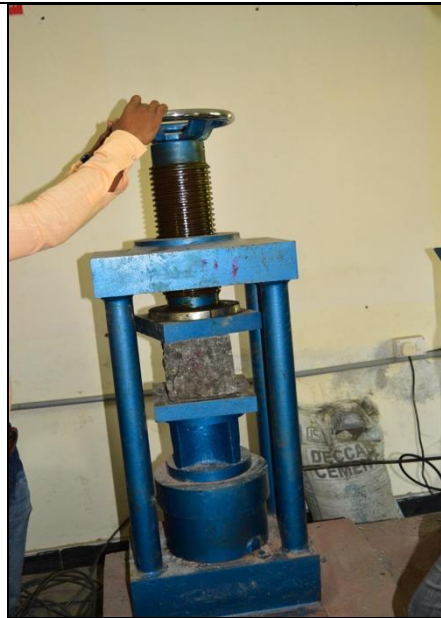
Fig 4.4: Compressive Strength Test Set Up for Cubes
