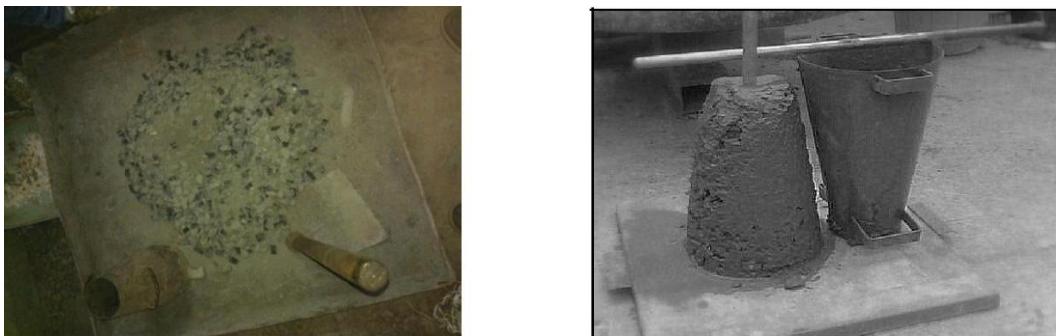
Fig 4.1: Process of Concrete Mixing and Slump Test
