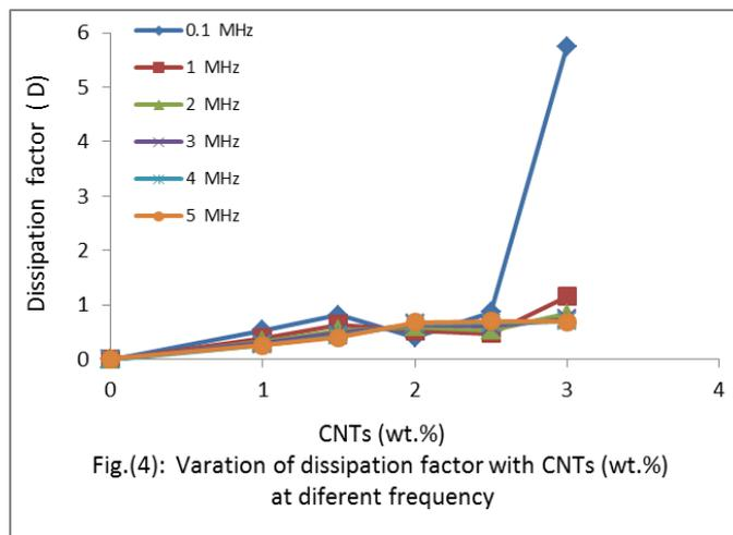
The dielectric loss of (PS) and its composites with different weight percentages(wt.%)of (CNTs) are obtained as a function of different frequencies given in figure (5).It is found that the dielectric loss of all these composites decrease at low frequency range (50Hz - 3MHz) and afterwards it nearly remains same at higher frequency range. Also it is clear in figure (6) at different frequencies when the weight percentage of (CNTs) increases dielectric loss of (PS) composites increases.
