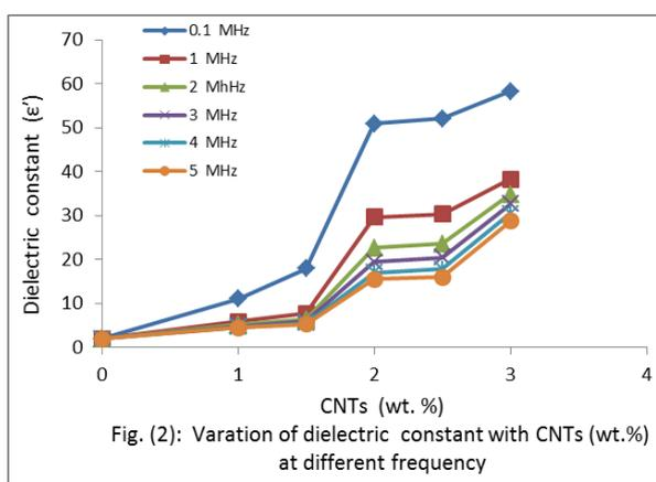
Fig. (2): Variation of dielectric constant with CNTs (wt.%) at different frequency
