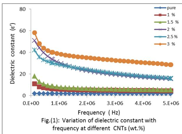
Fig.(1): Variation of dielectric constant with frequency at different CNTs (wt.%)
