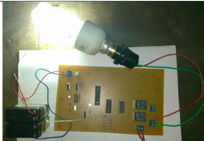
Fig.4: Proposed Hardware Design of RX part
