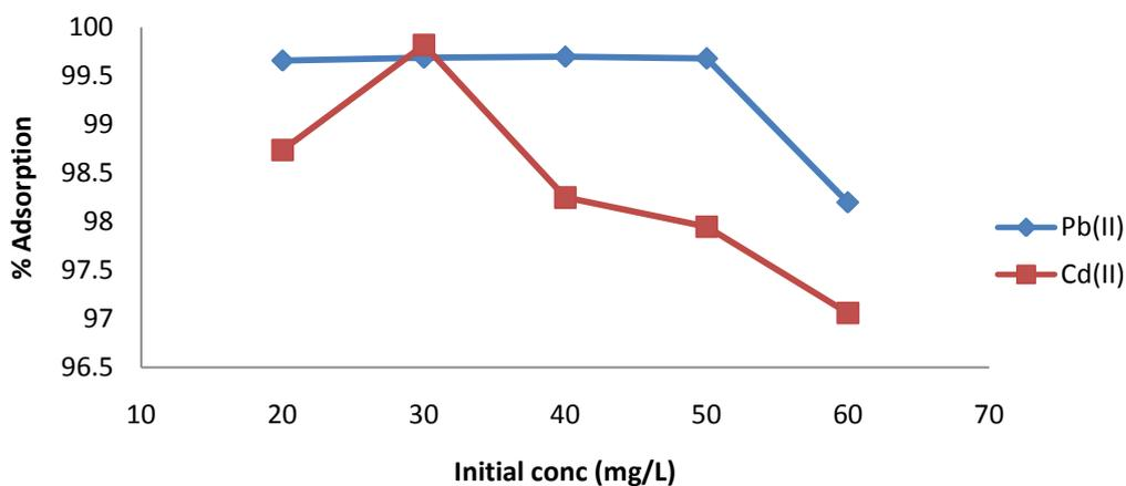
Fig 2. Effect of initial concentration on adsorption of P(II) and Cd(II) onto oil palm flower (Mass = 0.5g, volume = 100ml, time = 120min)
