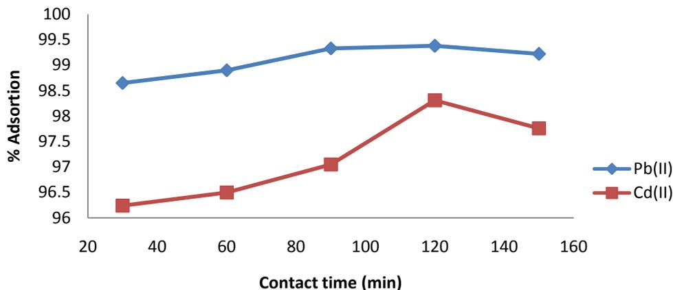
Fig 1. Effect of contact time on adsorption of Pb(II) and Cd(II) onto oil palm flower (Mass = 0.5g, conc. = 50mg/L, volume = 100ml)
