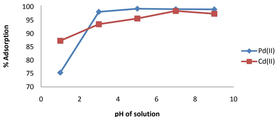
**Fig 3. Effect of pH on adsorption of Pb(II) and Cd(II) onto oil palm flower (Mass = 0.5g, conc. = 50mg/L, volume = 100ml, time =120min)**
