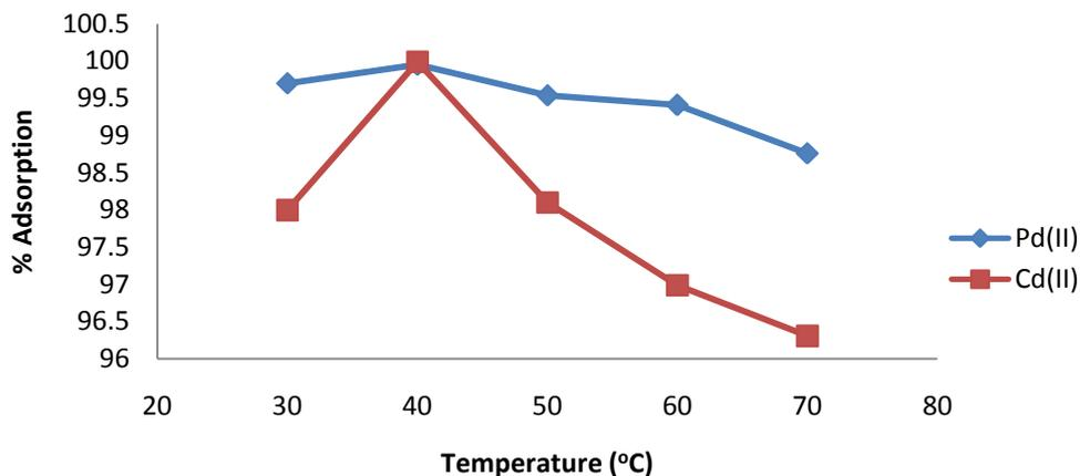
**Fig 5. Effect of temperature on adsorption of Pb(II) and Cd(II) onto oil palm flower**
