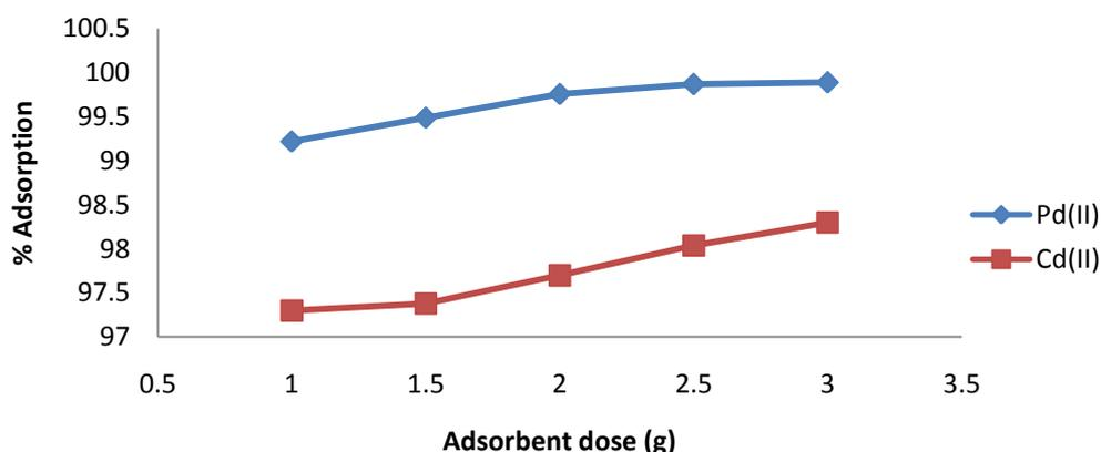
**Fig 4. Effect of adsorbent dose on adsorption of Pb(II) and Cd(II) onto oil palm flower (Conc. = 50mg/L, volume = 100ml, time = 120min)**
