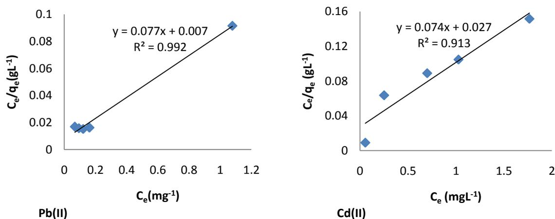
**Fig 6. Langmuir Isotherms for adsorption of Pb(II) and Cd(II) on oil palm flower**
