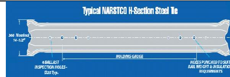
Fig 2 H-section steel tie
