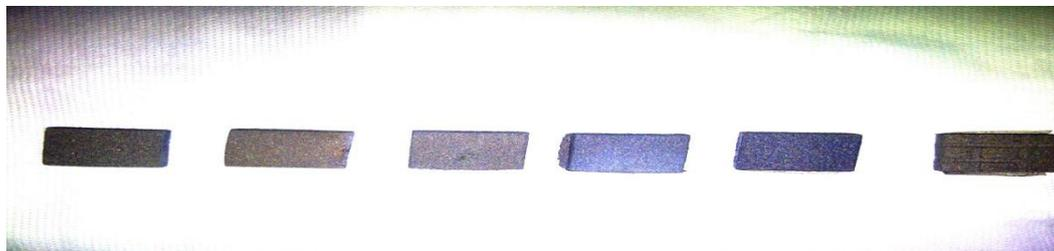
Fig (1) The samples after coatings with Ni-Al /ZrO<sub>2</sub>+Y<sub>2</sub>O<sub>3</sub>.
