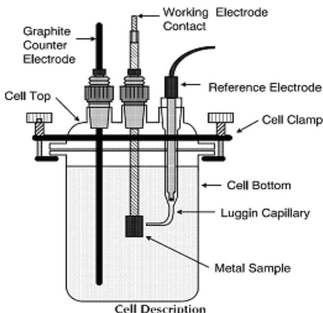
Fig(2): Schematic representation of a similar corrosion cell used for testing[13].
