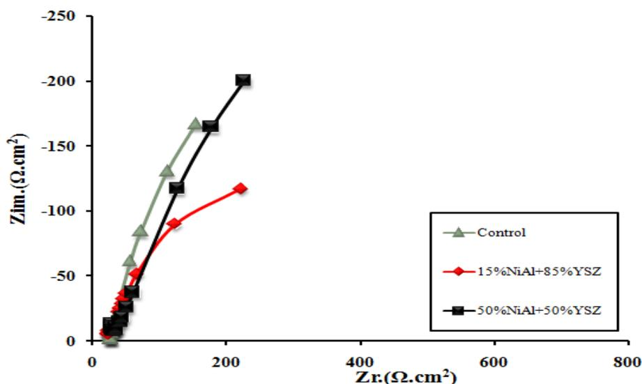
Fig 5: Nyquist diagrams of impedance spectrum for control (uncoated) and NiAl+YSZ coated carbon steel in crude oil .
