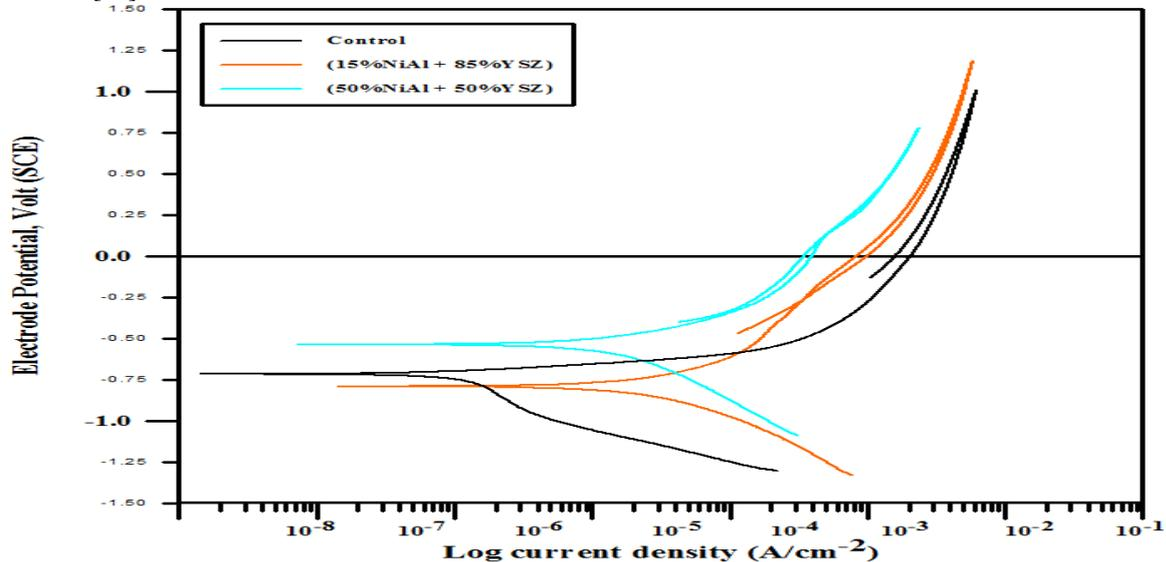
Fig 3: Cyclic polarization for the uncoated and (NiAl + YSZ) coated with different mixing ratios carbon steel in crude oil; Sweep rate 1 mV/sec.
