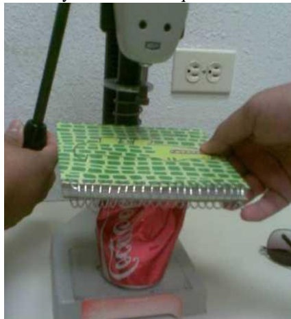
Fig:1.3Dynamometer used to crush a single can organized vertically
