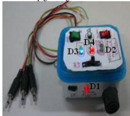
Figure 3- The overvoltage protection circuit in ON mode
