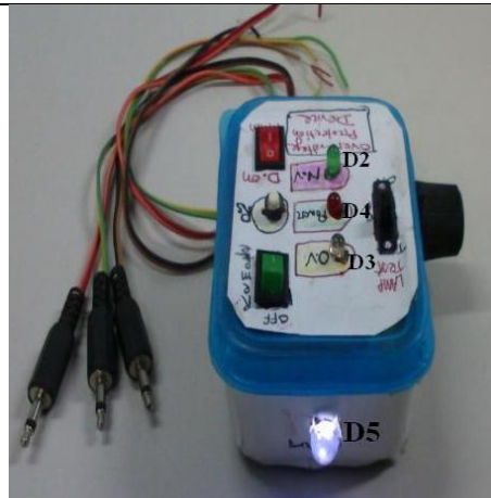
Figure 4- The overvoltage protection circuit in OFF mode
