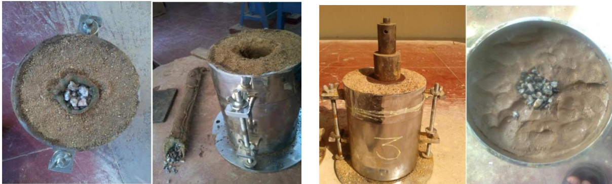
C] Geosynthetic encased granular pile D] prepared soil specimen E] granular pile installed in soft clay
