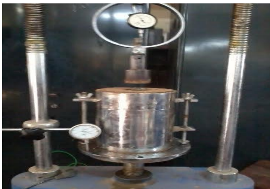
A] Test Setup using C.B.R Mould.
