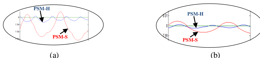
Fig.15 Oscillations of output voltage V_o in steady state at V_{ref} = 8\text{V}
