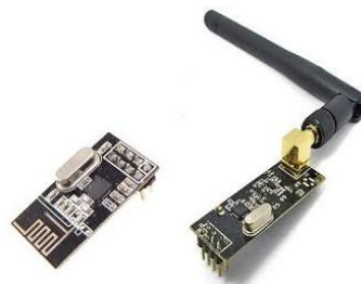
Fig. 1. The NRF24L01+ breakout board. The Left is the official design provided by Nordic Semiconductor, and the right is the version with Antenna amplifier for longer range.
