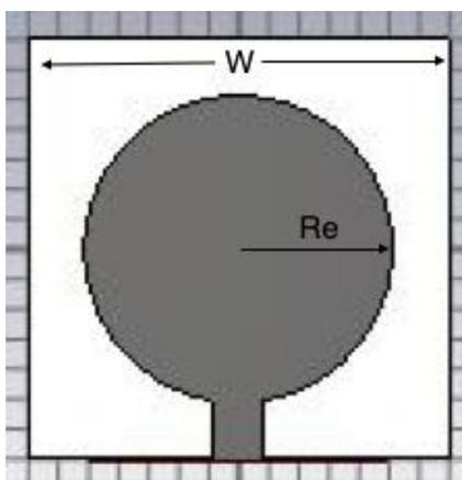
Figure 1: Circular Micro Strip Patch Antenna [11]
