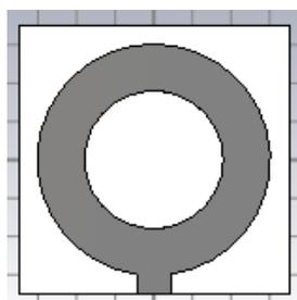
Figure 6: Slotted Circular Patch Antenna
