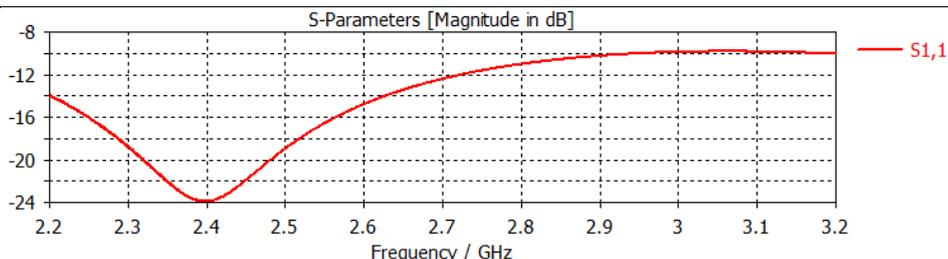
Figure 7: Return Loss Graph of Slotted Circular Patch Antenna
