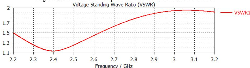
Figure 8: VSWR Graph of Slotted Circular Patch Antenna
