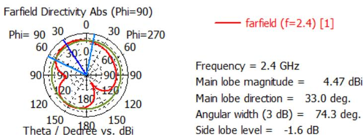
Figure 9: 2D Radiation Pattern of Slotted Circular Patch Antenna
