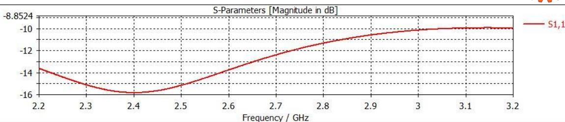
Figure 3: Return Loss Graph of Regular Non-slotted Circular Patch Antenna
