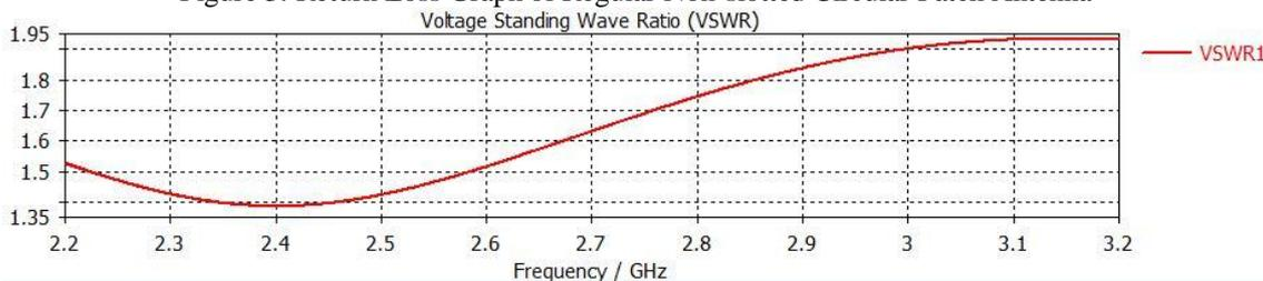
Figure 4: VSWR Graph of Regular Non-slotted Circular Patch Antenna
