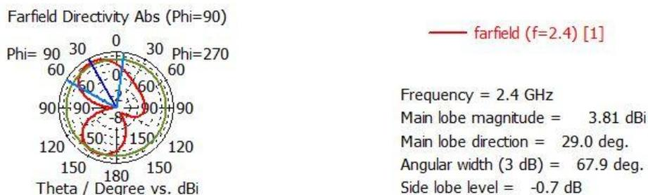
Figure 5: 2D Radiation Pattern of Regular Non-slotted Circular Patch Antenna
